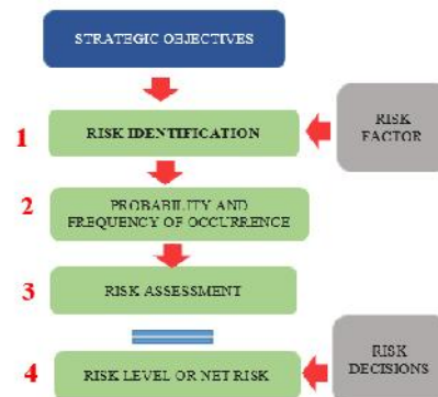
Fig 2. Phases of the elaboration of a risk matrix. Adapted from the Chilean Risk Prevention Experts Portal.
