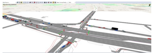
Figure 6: Model of the RCUT alternative, showing the bays for public transport stops/ Source: Own elaboration in Vissim.
